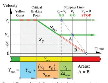
*Figure 4. Time model including vehicle deceleration traversing the minimum stopping distance.*
