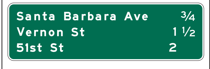
Figure 2E-31. Interchange Sequence Sign
